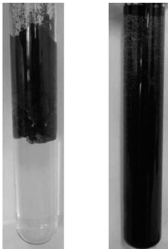
Figure 1 The dispersing stability of unmodified and plasma-treated GTR in water.
